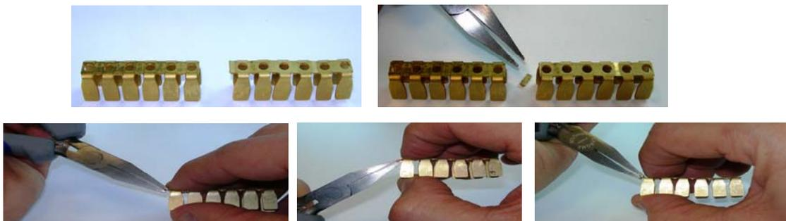
4. Cutting the insulating parts with screws inserted to obtain the number of poles required to complete the jumpers and proceed with the assembly as shown in the sequence below
