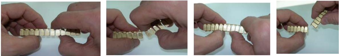
3. Remove the small piece with a witness who remains in one of 2 parts. (This operation is only to ensure the insulation distance in the case apply jumpers contiguous in sequence and to facilitate the placement of a separator terminal if the bridge is positioned at the last terminal of a group.)
