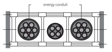
6. In case that is not possible to lay the cables as described under â, in order to lay several multi core high flexible cables with an outer diameter < 10 mm, we recommend the use of a guiding tube, in which these cables should losely laied. This tube is than integrated into the drag system. The cross section of this tube has to be much larger as the sum of the cross sections of the cables. For the free movement of the flexible energy conduits, the guide or divider stays must be installed.
