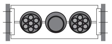
1. Where flat and round cables are mixed in one drag tray, then these should be installed loosely next to one another. The guide stays should be installed between the cables laid side by side. Try and avoid placing different sizes of round cables next to one another. Due to the limited space relationship cables arranged one above the other, frame stays are to be installed.
