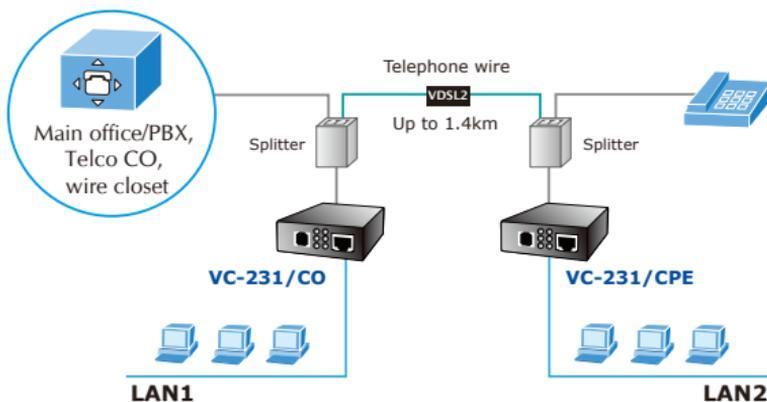
Refer to the following procedures to set up the VDSL2 Bridge LAN to LAN connection.
