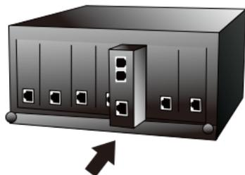
**Step 3:** Attach a rack-mount bracket to each side of the Converter Chassis with supplied screws attached to the package.
