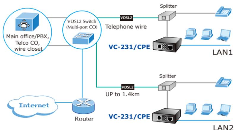
Refer to the following procedure to set up the VDSL2 Bridge to IP DSLAM connection.
