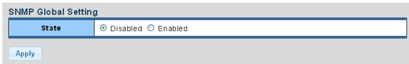
Figure 4-2-21: SNMP Global Setting Page Screenshot
