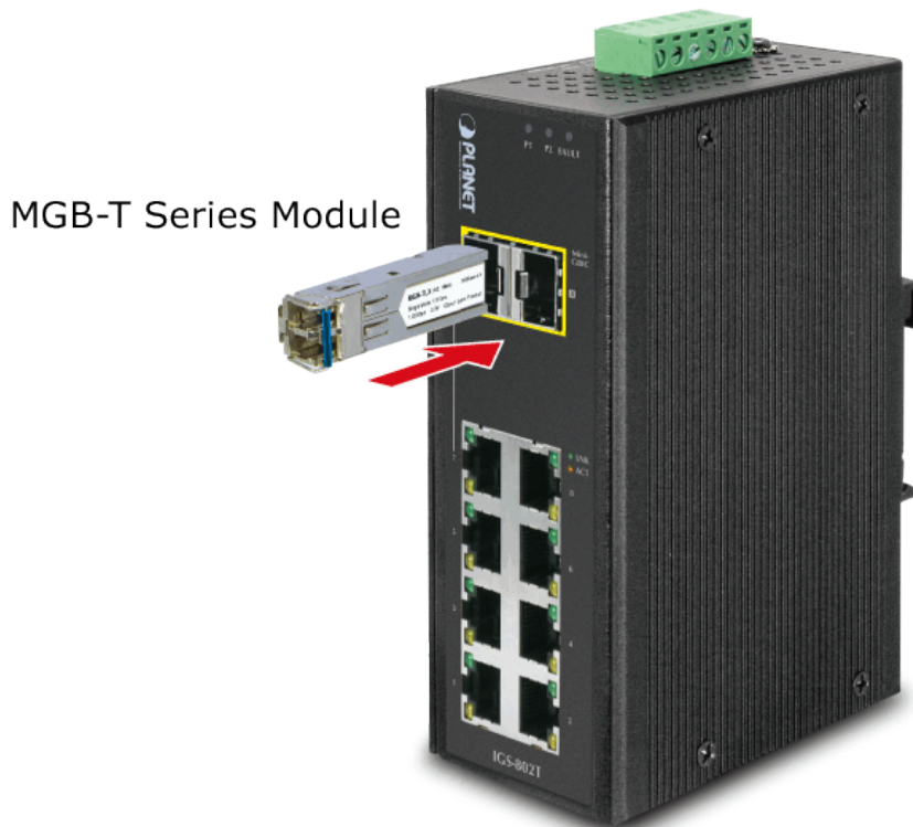
Figure 2-2-4a: Plug in the SFP Transceiver
