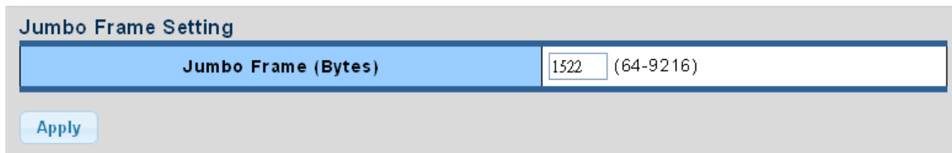
Figure 4-3-11: Jumbo Frame Setting Page Screenshot
